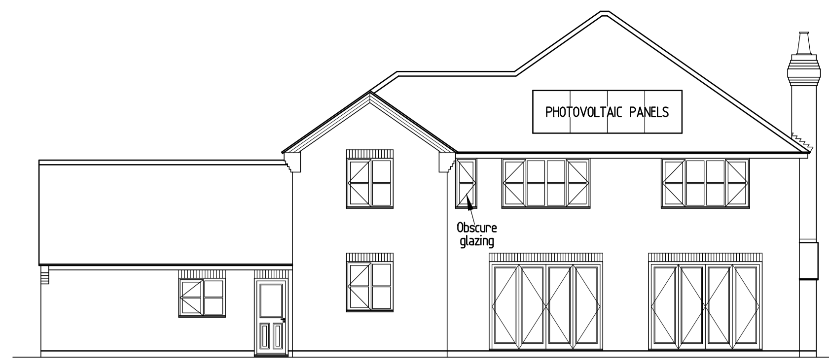
PROPOSED WEST ELEVATION Scale 1:100
