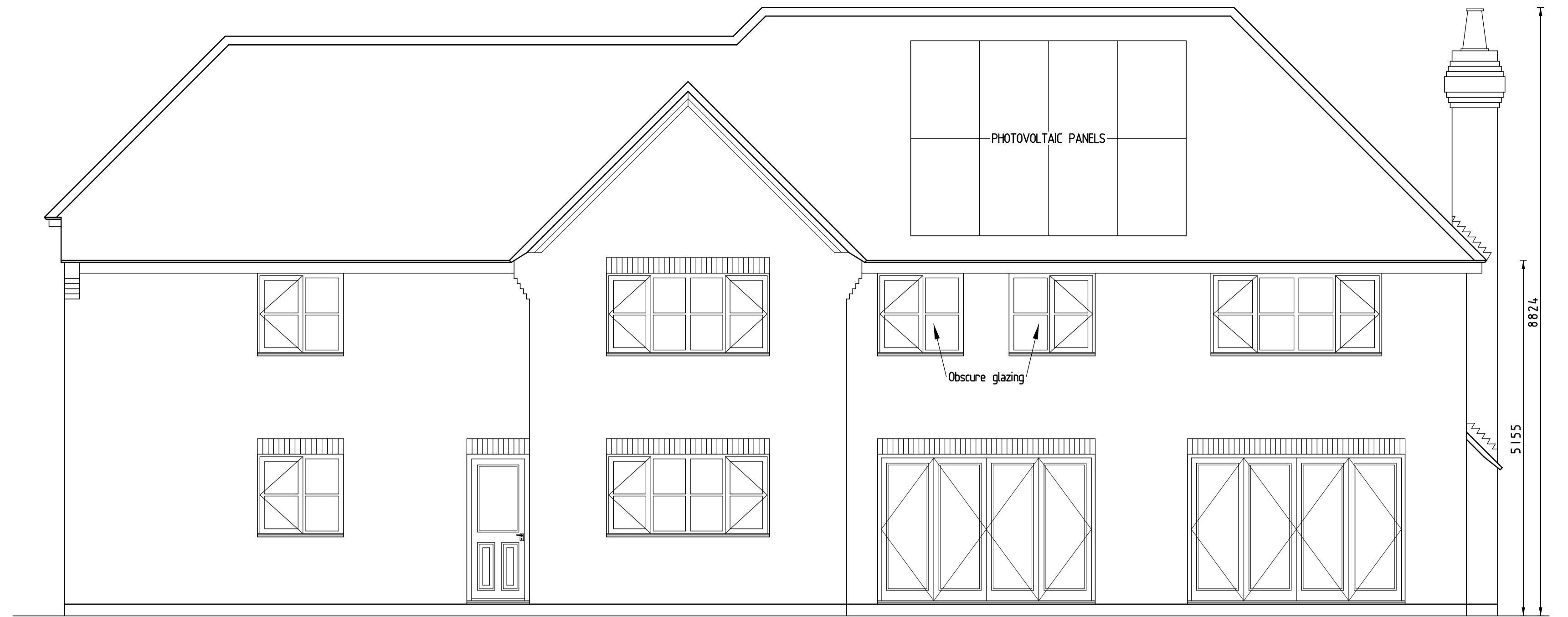
PROPOSED WEST ELEVATION Scale 1:50
